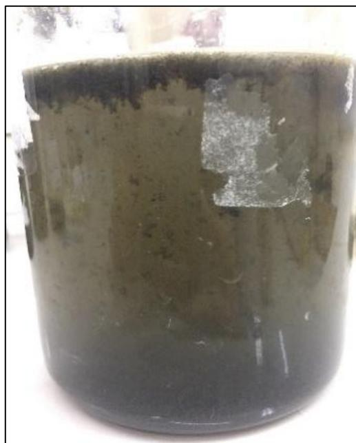
**Figure 6** Floc formation with Polyacrylamide concentration of 200 mg/L
