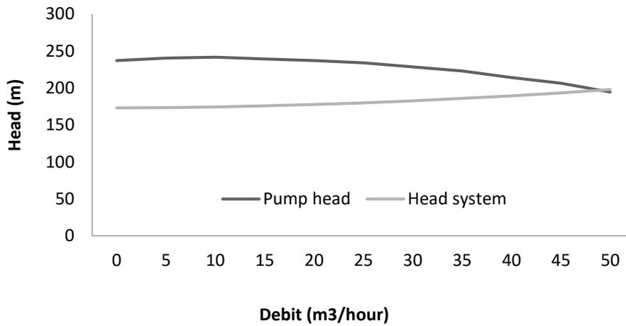
Figure 4 The curve of clean water transfer pump
