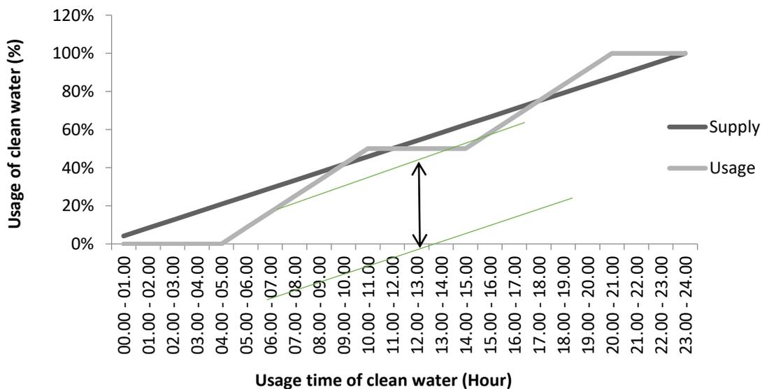
Figure 3 The graph of cumulative supply and cumulative usage of bottom reservoir
