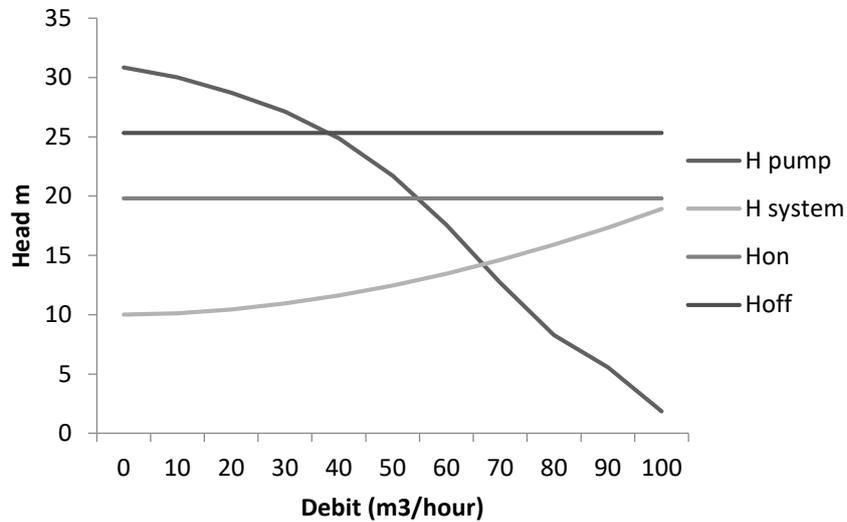
Figure 6 The graph of clean water booster pump
