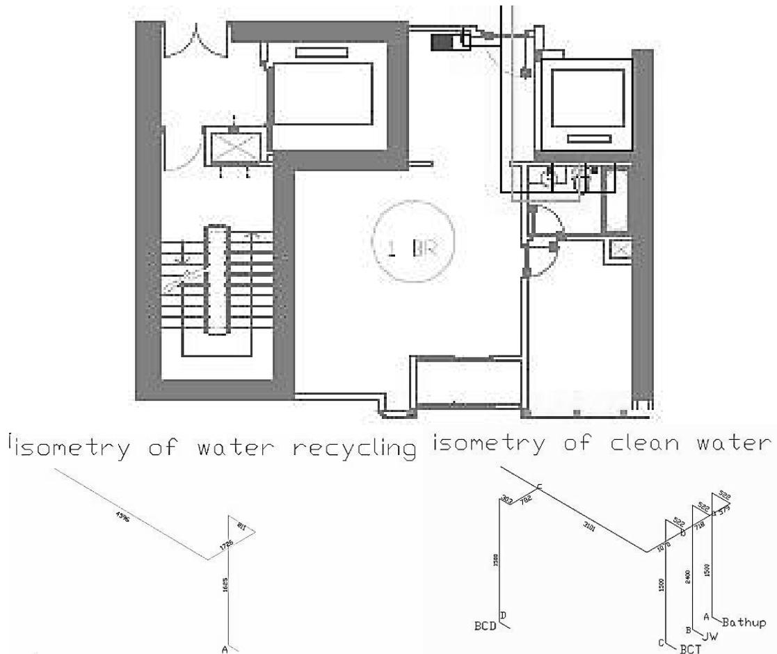
**Figure 1** The lines and isometrics of clean water and recycled water of residence with 1BR-type
