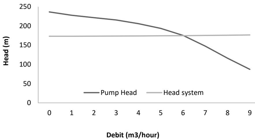
Figure 5 The curve of recycled water transfer pump
