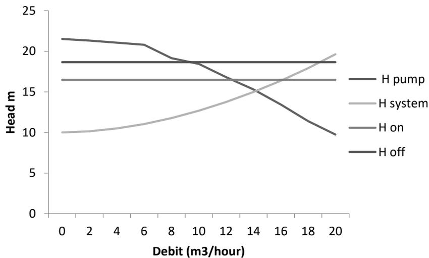
Figure 7 The graph of recycled water booster pump
