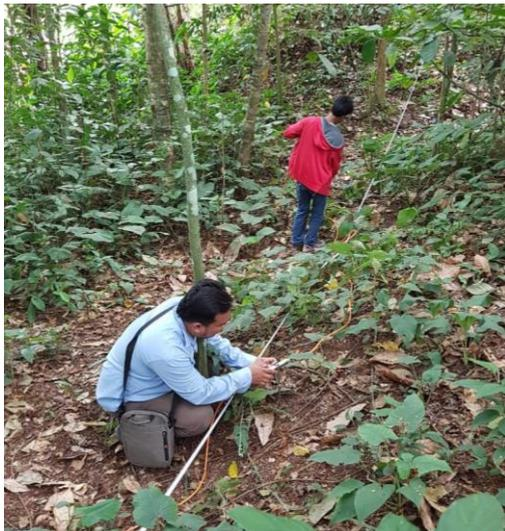
Figure 1. Measurement survey of the groundwater depth using geoelectrical method
